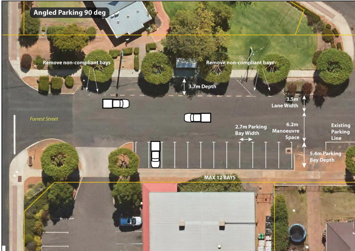
Figure 1: Parking at 90 Degrees
