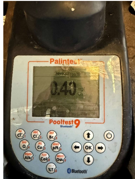
Tap water chlorine test (DPD1)
