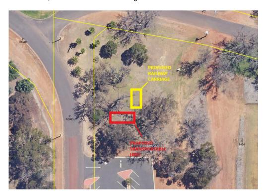
The Transportable Unit is 12m long, 4.37m wide and 2.9m high. The floor area consists of two (2) meeting rooms, two (2) storage rooms and includes a wash basin. The roof is constructed using zincalume steel sheeting. It is proposed that a mural is painted on the walls of the Transportable Unit, to enhance its appearance to the street frontage.
