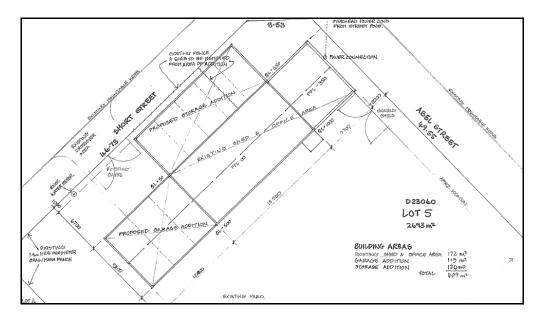
The storage shed is 6.7m X 18.5m ( $124m^2$ ), with a wall height of 3.1m. The workshop is 9.1m X 12.4m ( $113m^2$ ), with a wall height of 5m. Both structures are
